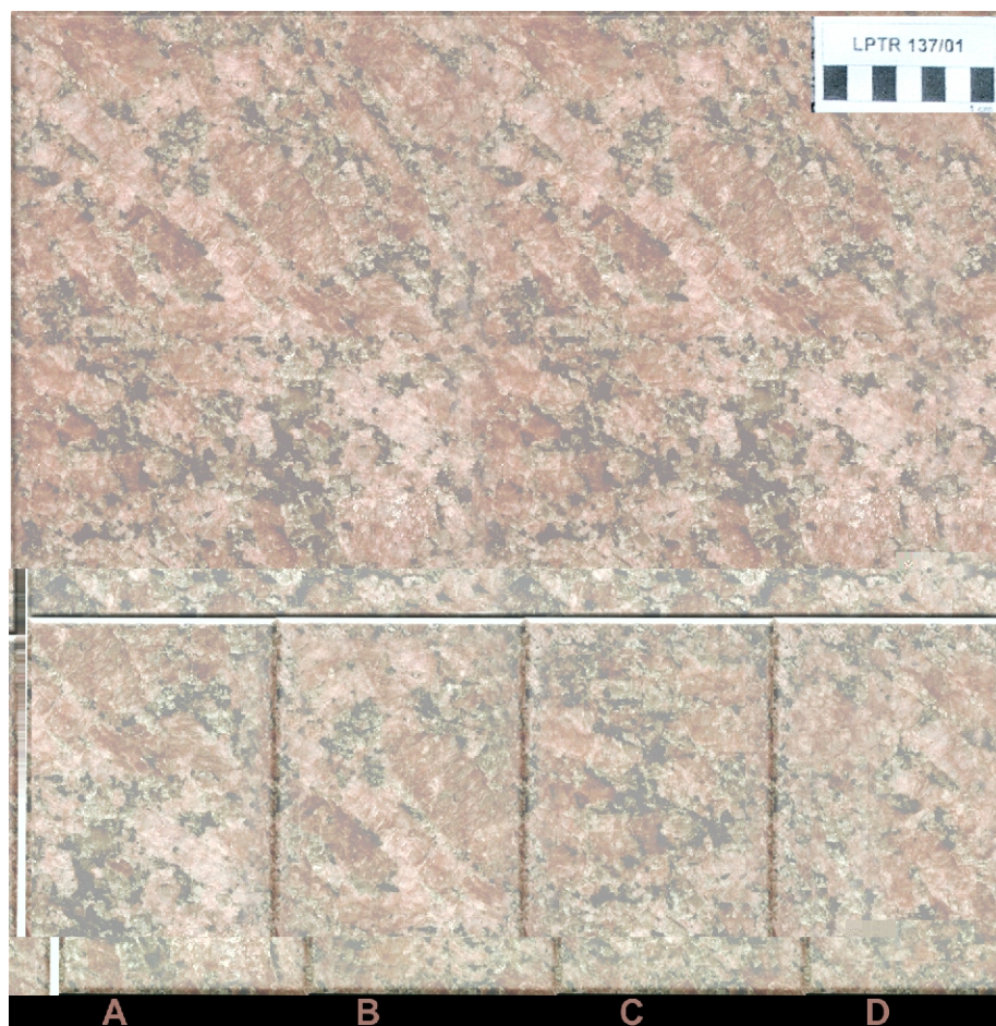
PICTURE 1 - Samples used in the artificial light and water exposure test.
